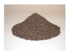
Almandite garnet is a high hardness, high density granular filter media. It can be used extremely effectively as the lower strata in a dual media filter bed. Its high specific gravity as well as its chemical and abrasive resistance makes almandite garnet ideal for filtration.
